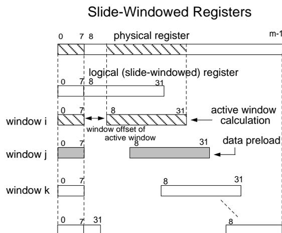
Figure 6. Schematic graph of slide-windowed registers.
