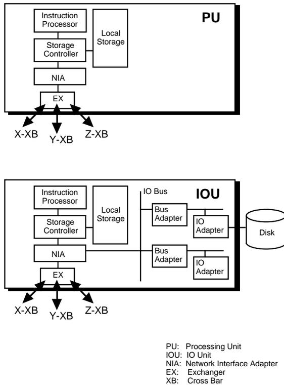
Figure 9. Schematic configuration of Processing Unit(PU) board and IO Unit(IOU) board of CP-PACS.
