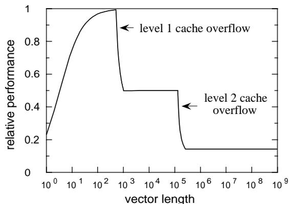
Figure 5. Performance of a RISC processor in a large scale scientific calculation.
