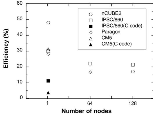
Figure 15. Efficiency in terms of the ratio of the sustained speed to the theoretical peak speed[19].
