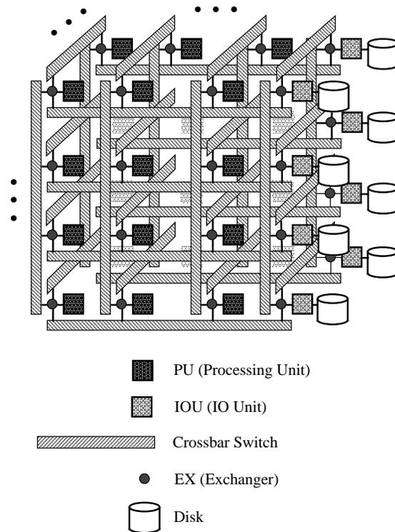
Figure 10. System configuration of CP-PACS.
