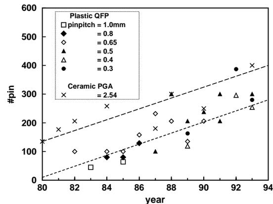
Figure 4. Evolution of the number of pins. (From "Nikkei Electronics" August 2, 1993.)
