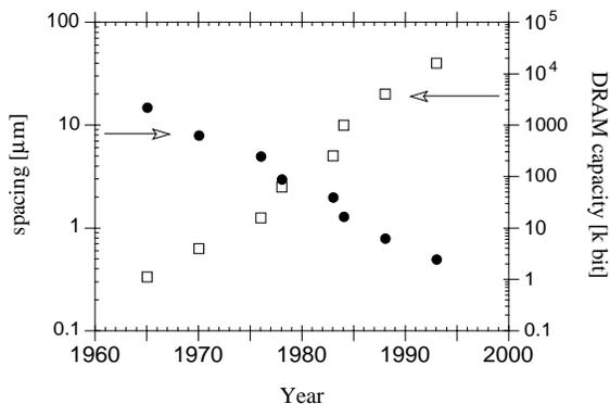
Figure 3. Development of minimum spacing of LSI and capacity of DRAM.
