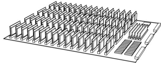
Figure 13. Mechanical design of a mother board of the 0.5-Tflops project.
