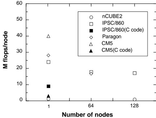
Figure 14. Sustained speed in terms of flops/node of commercial parallel computers for the conjugate gradient matrix inversion with staggered quarks[19]. The results for Paragon and CM5 are preliminary.
